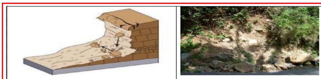
Figure 2.1: Schematic view rock fall ((Highland et al, 2008) and photo of rack fall in Samigaluh Disrtict in 2011(Eko Setya N, 2011)
