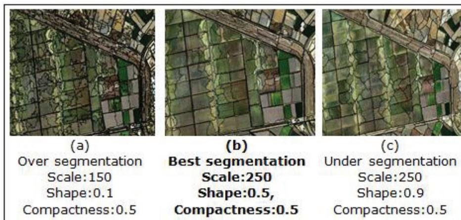
**Figure 12: Segmentation result using different parameters.**
