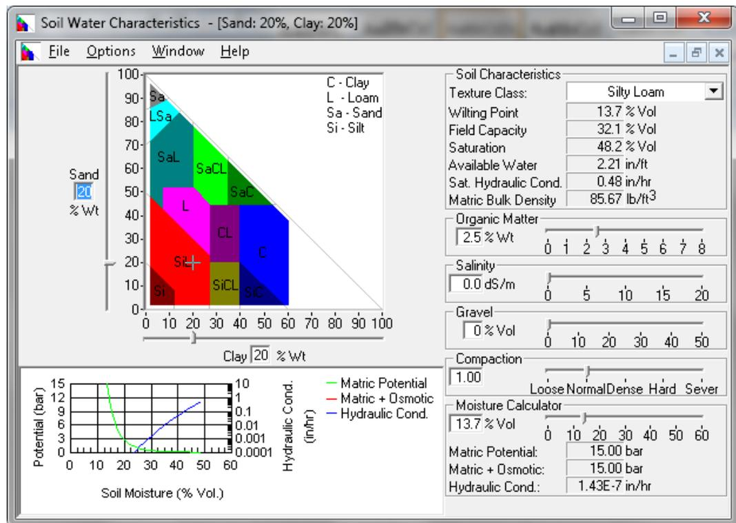
Figure 2-4. Soil water characteristic program.
