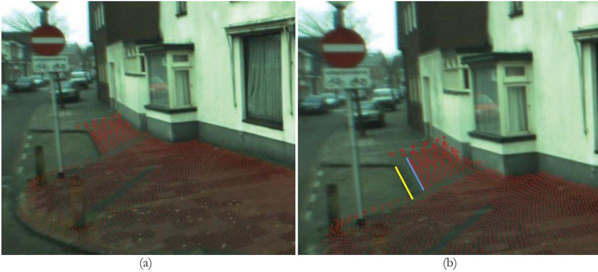
Figure 4.9 The co-registration between image and the selected plane feature on the ground (a) is the back-projection result using the original EOPs; (b) is the result using corrected EOPs
