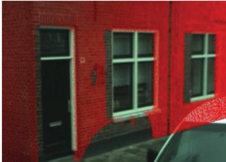
Figure 4.3 The back-projection result of direct geo-referenced data (red points are the back-projected laser points)
