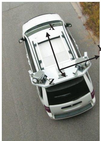
Figure 4.2 The body frame coordinate system of LYNX system
