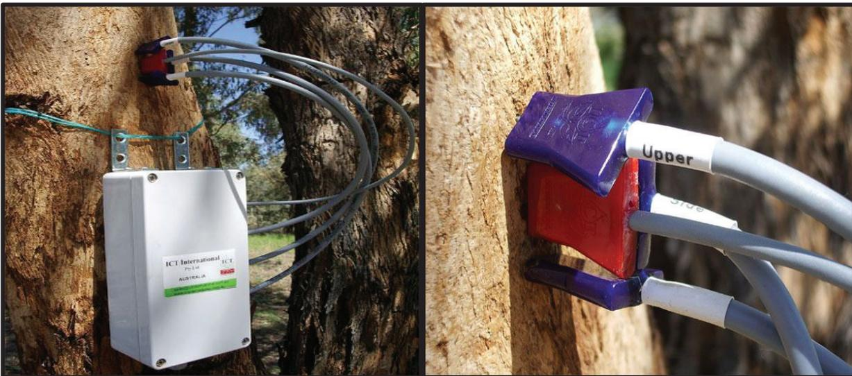
Figure 2: Heat Field Deformation for measuring Sap flux density (Source: <http://www.ictinternational.com.au/hfd.htm>)
