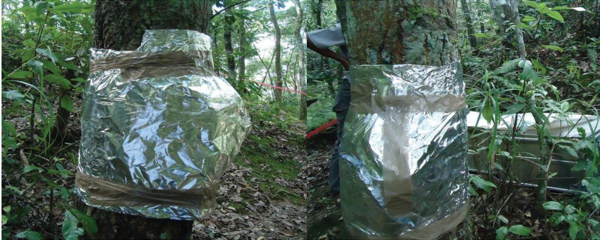
Figure 7: Thermal insulation provided in the sensors for preventing from NTG
