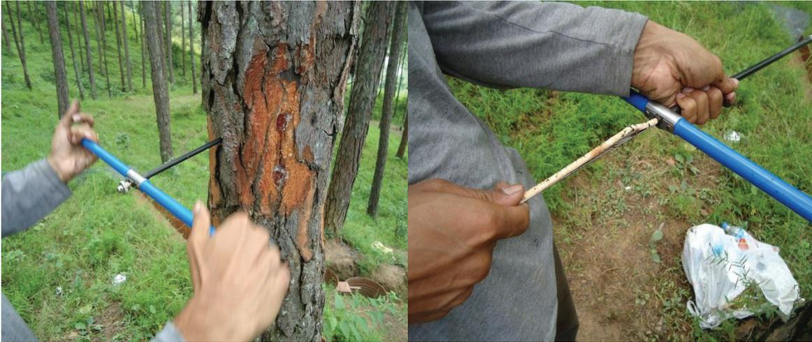
Figure 9: Tree boring for sapwood area determination (left) and obtain sample (right)
