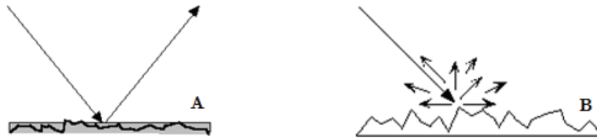
Figure 3: (A) Specular reflection from flooded area (B) Diffuse reflection from non-flooded area Source: Centre for Remote Imaging, Sensing and Processing (CRISP)
