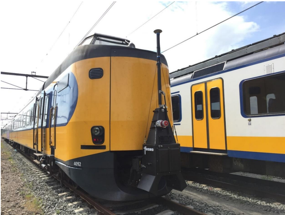
Figure 1-1 - Mobile Laser Scanner mounted on the Rail (Source -Fugro )
