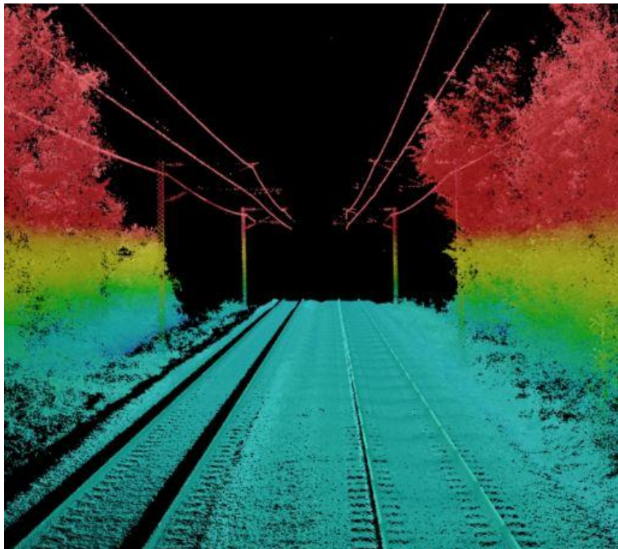
Figure 3-1 MLS point cloud dataset of a railway environment (points are colored based on their elevation)
