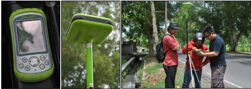
Figure 24 Field survey measurement using DGPS RTK Triumph-1 JAVAD GNSS
