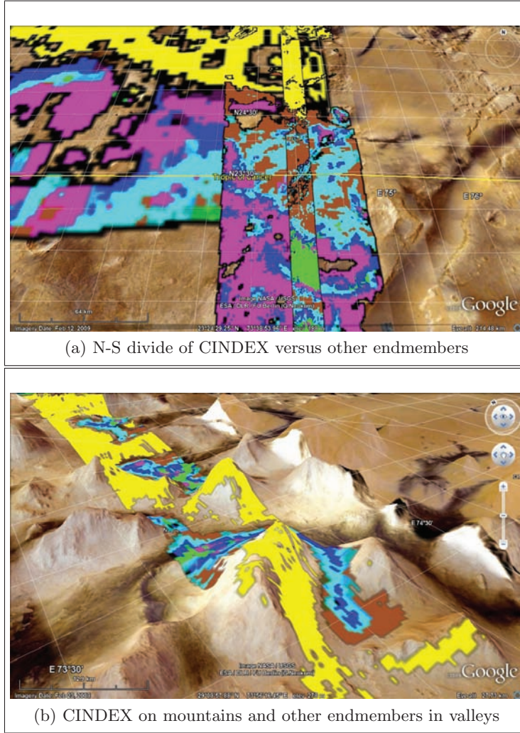
Figure 3.19: Details of the spectral angle maps overlaid on Google Earth/Mars. In 3.19a, patches of CINDEX in the North are coherent across resolutions and patches of LCPINDEX in the South are sometimes coherent (occurring in the same geographical areas) between 3047_5 and 0232_2. Overlaid images have black borders to highlight the overlapping resolutions. CINDEX and the other endmembers occupy distinct geomorphological units in the 3047_5 overlay in 3.19b. Vertical exaggeration \times 3 .
