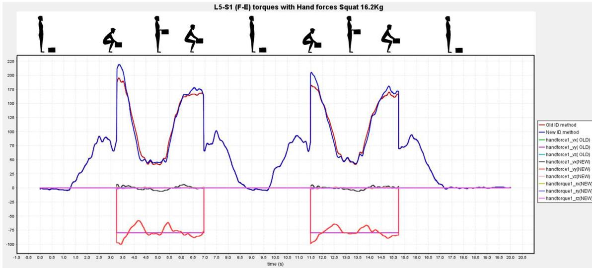
Fig D.1. L5-S1(F-E) torques for Squat 16.2 kg condition
