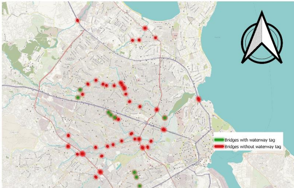
Figure 5.18: Tag completeness for Bridges and overpasses highways crossing.
