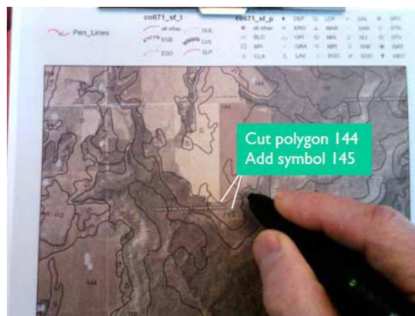
Figure 6. Using the digital pen for a soil survey (Source: (Price, 2010)).
