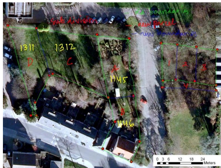
Figure 19. Boundary corners to identify parcel are marked using points (red) and connected using “imaginer lines” (green).
