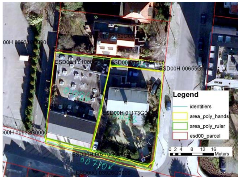
Figure 25. Comparison between the drawing (yellow by free hand, green by ruler), the existing cadastral map (red) and the aerial photo.
