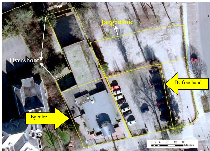
Figure 22. Results of two methods of drawing lines (by free-hand and by ruler).
