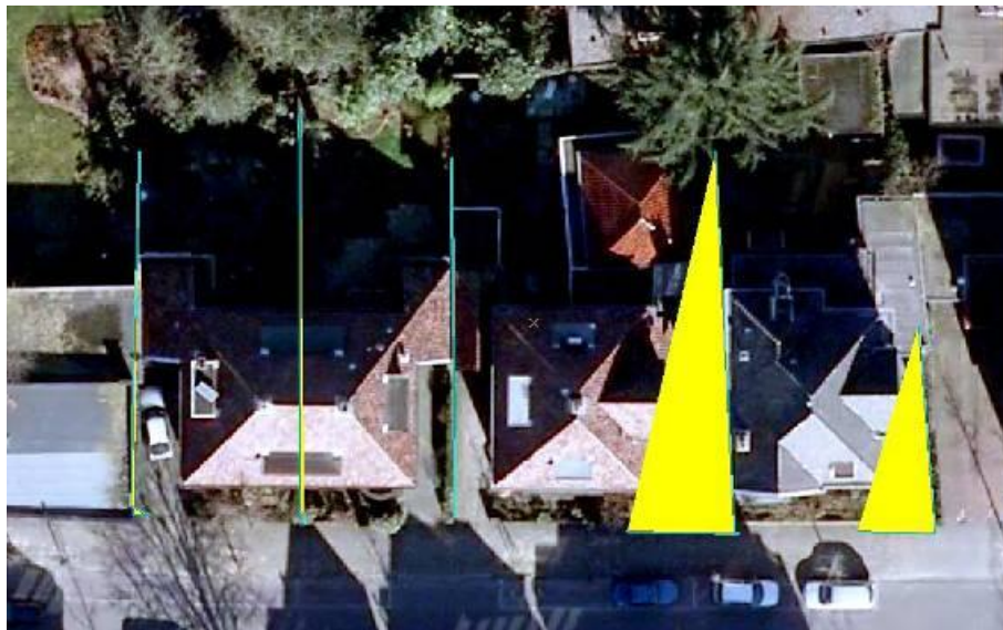
Figure 17. Incomplete parcels (yellow) caused by incompleteness of recording the boundaries (blue).
