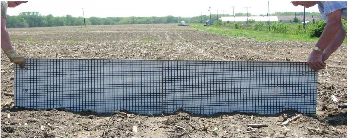
Figure (2-8) The 2-m grid board placed in soil surface for characterization of surface roughness
