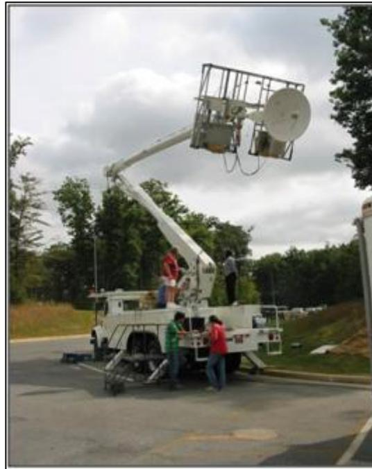
Figure (2-2) The truck mounted radar/radiometer system called ComRad
