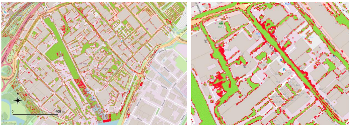
(a) Overview of De Pijp (b) Close-up of Wijkermeerweg Figure 13 - Agreement and disagreement on flooded area of De Pijp for bui09
