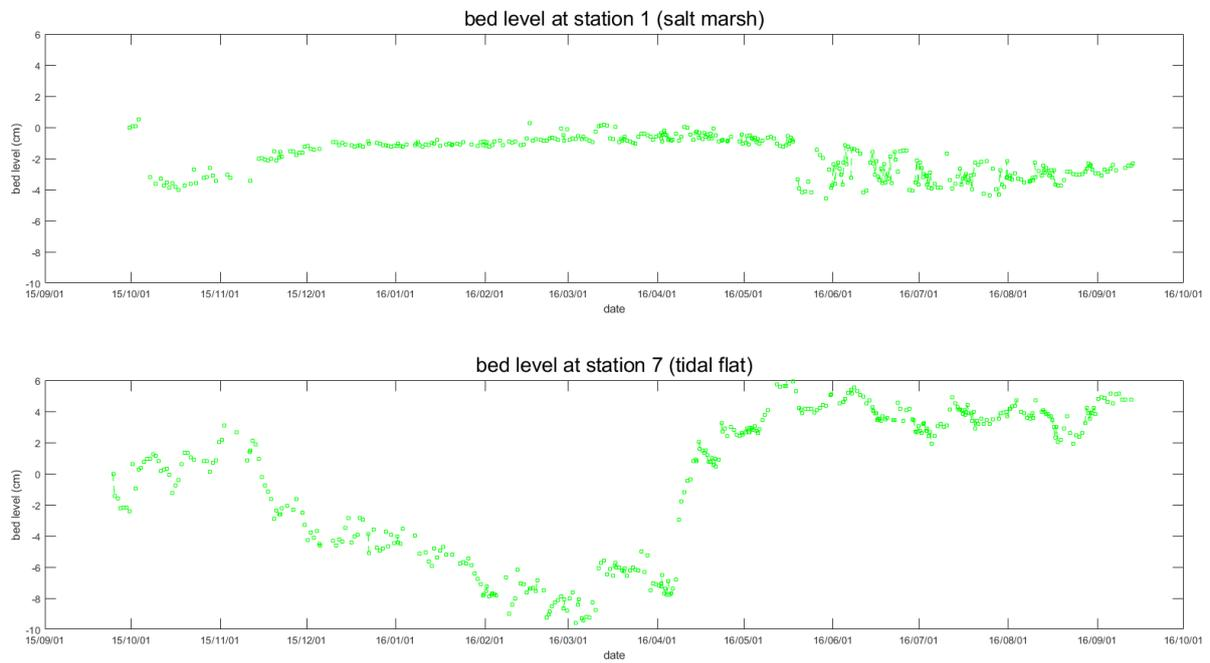
Figure 17 bed level change graph at each station in Site 2
