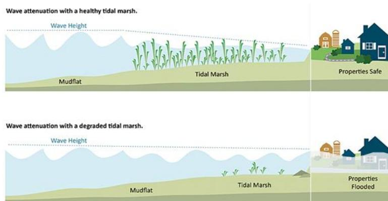
Figure 10 Wave attenuation with a healthy tidal marsh (Governor's office of storm recovery, 2016)
