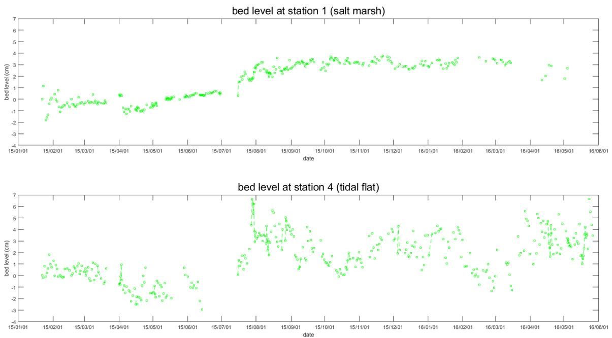
Figure 18 bed level change graph at each station in Site 4
