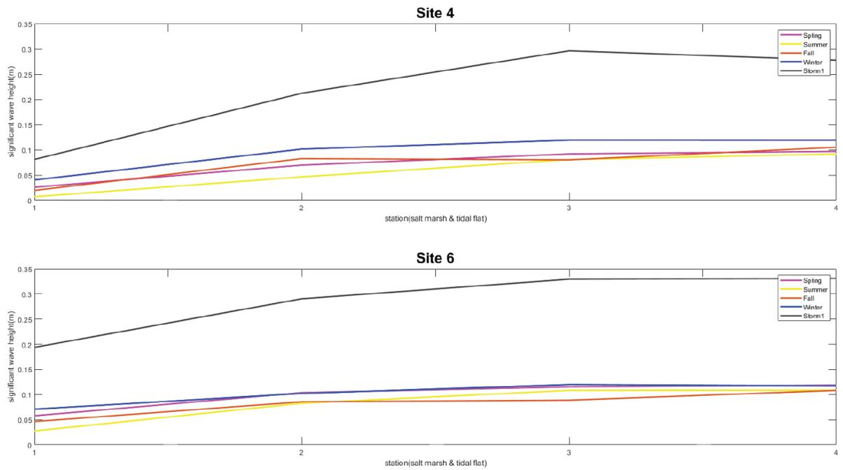
Figure 23 Significant wave height during each season and stormy period (Site 4 & 6)
