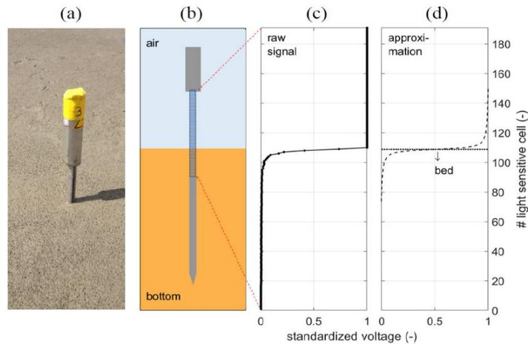
Figure 1 (a) represents picture of a SED-sensor, (b) represents schematization of a SED-sensor, (c) represents raw voltage signal from a SED-sensor and (d) represents voltage signal without noise
