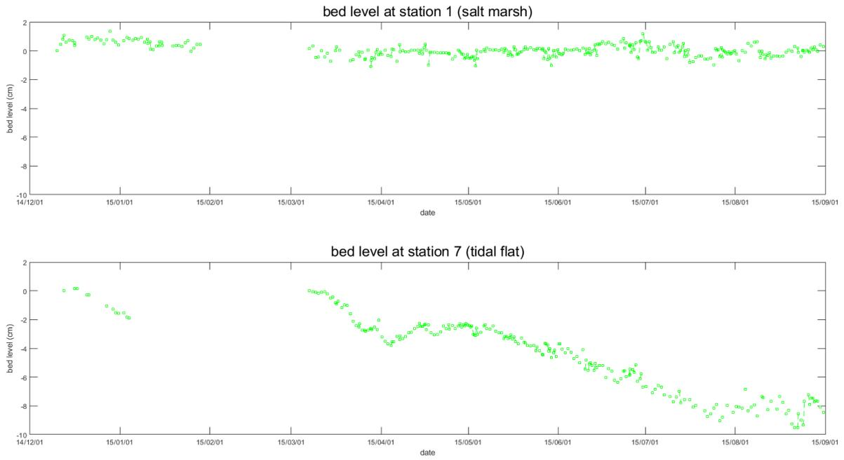
Figure 19 bed level change graph at each station in Site 5
