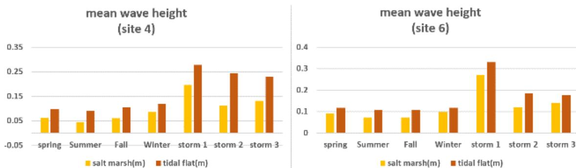
Figure 11 mean wave height at site 4,6
