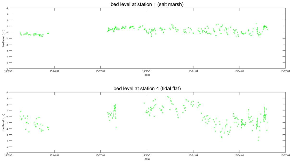
Figure 20 bed level change graph at each station in Site 6
