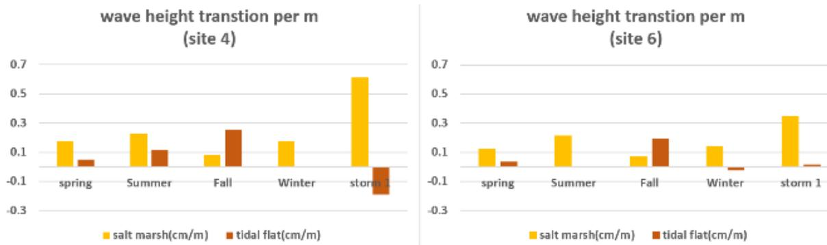
Figure 12 wave height transtion per m at site 4,6
