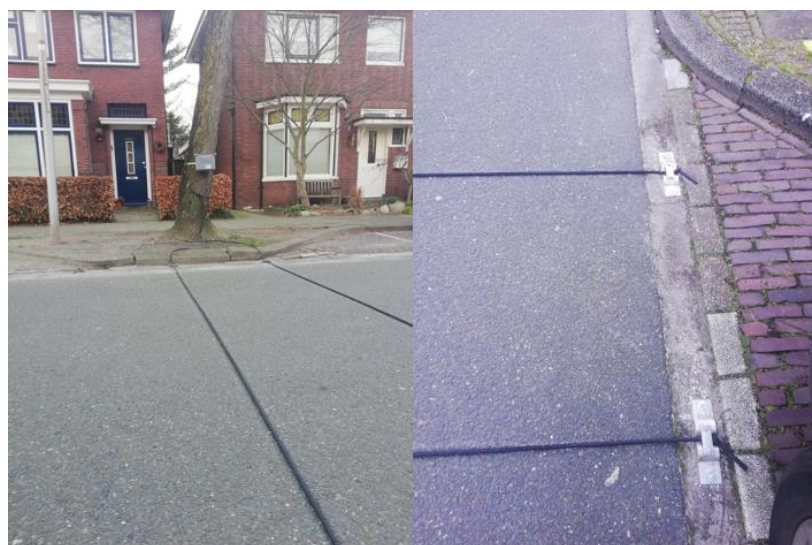
Figure 2 - Left: road tubes installed on a road. Right: end of the tubes drilled into (the edge of) the road surface
