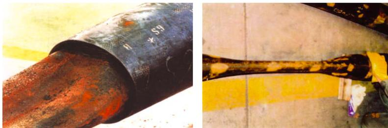
Figure 1.1: Local buckling of a steel casing used in oil/gas well applications (Dvorkin and Toscano, 2003)
