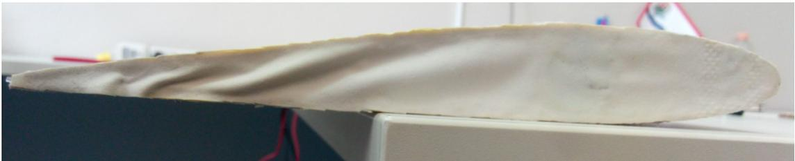
**Figure 6.1:** The wing in its downwards actuating position.
