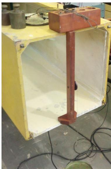
**Figure 5.6:** The configuration used to calibrate the drag sensor. The pulley converted the vertical load of the weights on the scale to a horizontal load.
