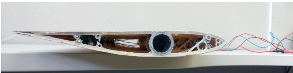
**Figure 4.11:** Bending test performed of frame with wood skin.
