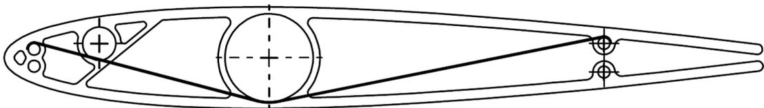
**Figure 1:** Drawing of one of the ribs with one SMA wire attached. The antagonistic wire is attached in the same way, but mirrored over the horizontal symmetry axis and slightly off-set in depth direction, to prevent contact with the opposing wire.
