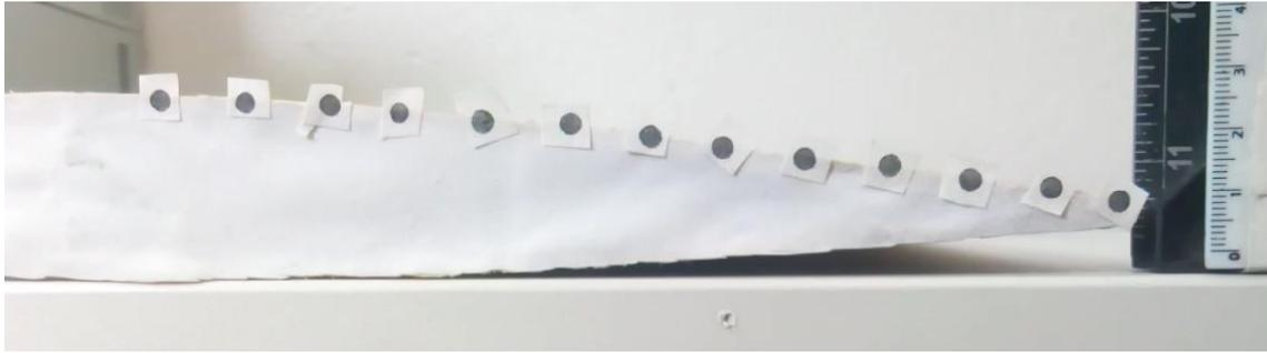
**Figure 5.1:** One of the images used to analyse the upwards movement of the wing.
