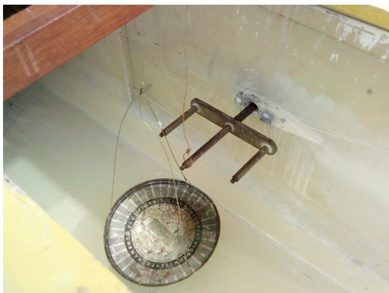
**Figure 5.5:** One of the scales used to calibrate the lift sensors.
