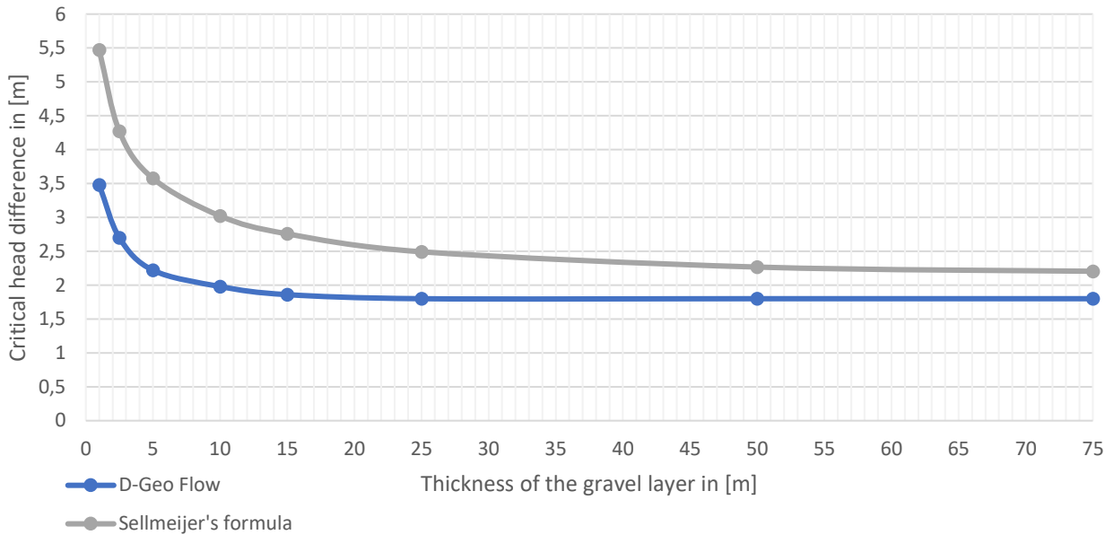
Figure 24. Effect of the thickness on the critical head difference
