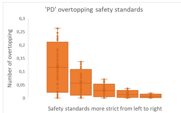
Figure 13 - Effect of safety standards on overtopping frequency of 'PD'
