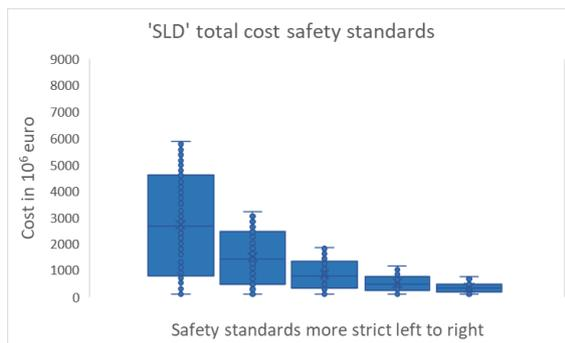
Figure 14 - Effect of safety standards on total cost of 'SLD'
