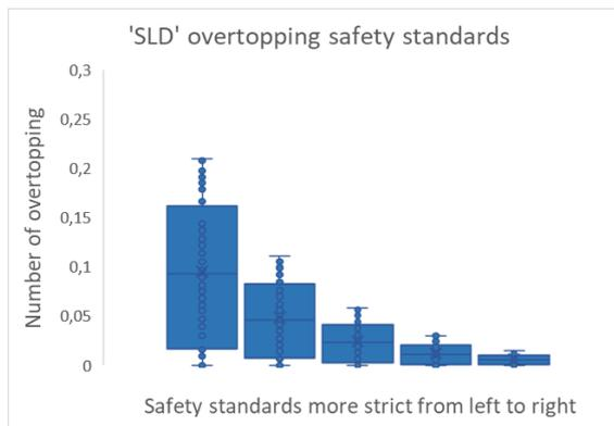
Figure 12 - Effect of safety standards on overtopping frequency of 'SLD'
