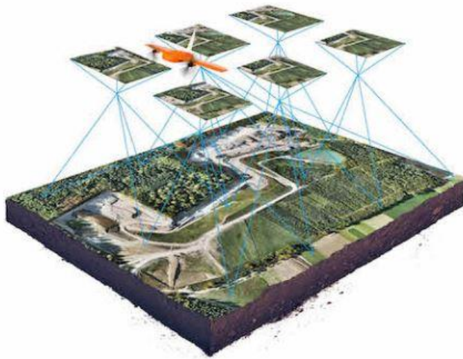
Figure 1: Example of UAV Photogrammetry data acquisition (source: www.wingtra.com )
