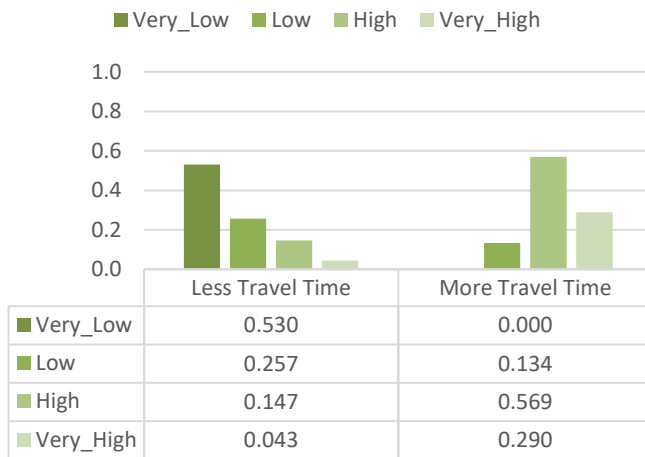
Figure 40: CPT table showing the effect of Travel Time on ‘Traffic Intensity’ – AMS, 2019
