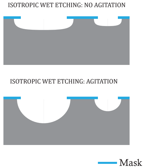
Figure 2.2: Schematic of agitation effects on isotropic wet etching.
