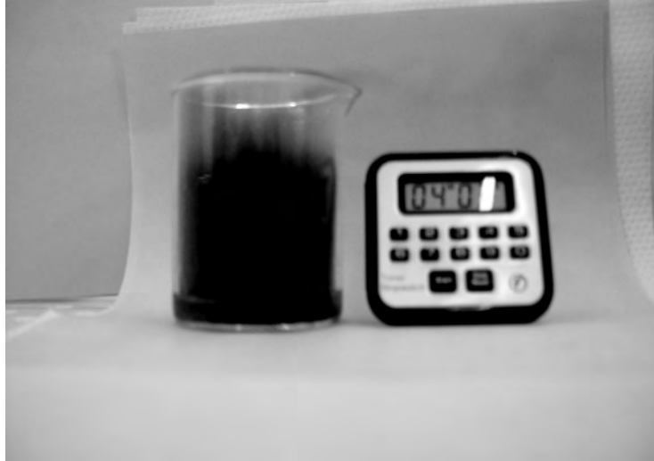
Figure 2.1: Photograph of the runaway reaction by 12.5 ml of an HNA solution with \text{HF}:\text{HNO}_3:\text{CH}_3\text{COOH} = 2:4:4 , on a 35\text{ mm} \times 35\text{ mm} silicon piece. [31]. The dense brown \text{NO}_2 gas formed and the timer shows the time after reaction started.
