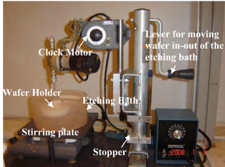
Figure 2.11: Agitation setup for UEA. The wafer holder and stirrer bar can rotate in opposite direction [50].
