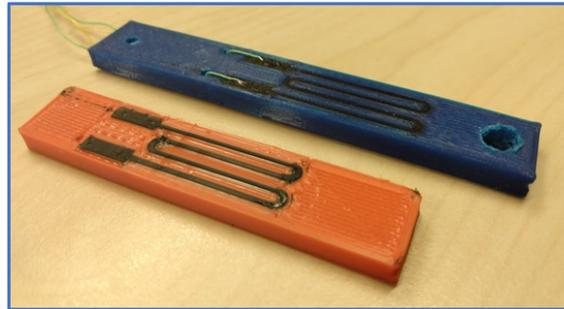
**Figure 3.2:** Orange: TPU with ETPU sensor; Blue: PLA with Proto-pasta sensor, which is used for the sensor characterisation in section 5.1
