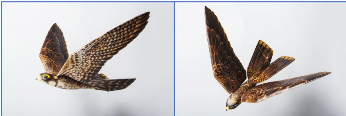
**Figure 1.1:** State-of-the-art mechanical bird called the 'Robird', which is able to fly with a pilot. ©Aerium and Clear Flight Solutions
