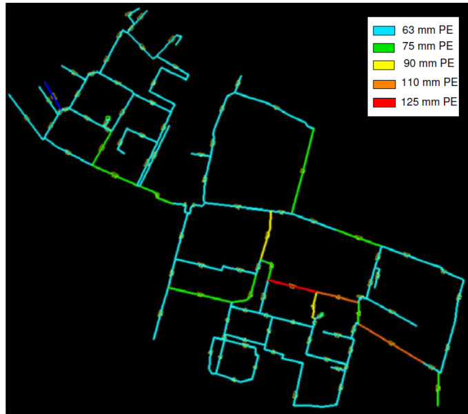
Figure 2.8: Schematic of part of a gas distribution grid in Arnhem, Netherlands. Varying colors indicate the difference in pipe diameter, as indicated by the legend (Dertien, 2014)
