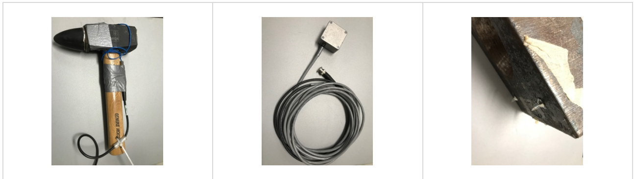
Figure 6.3: Impact hammer (left), acceleration sensor (middle), steel block with spikes (right).
