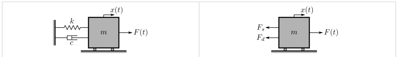
Figure 4.1: Viscously damped mass-spring system subjected to external excitation [3].
