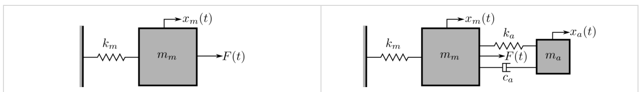
Figure 4.2: Dynamic vibration absorber [3].
