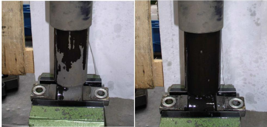
Figure 18: Damper leakage failure
