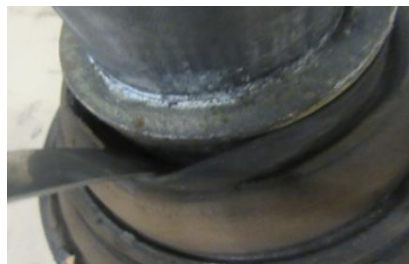
Figure 13: Rubber loose in Primary suspension
