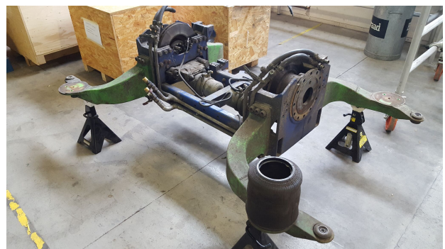
(b) Testbus subframe removed
