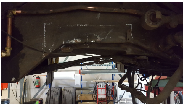
(c) Determining the cutout in the chassis
