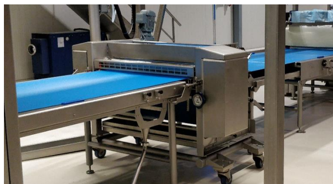
Figure 2.10: Example of a modular machine on wheels installed on the production line
