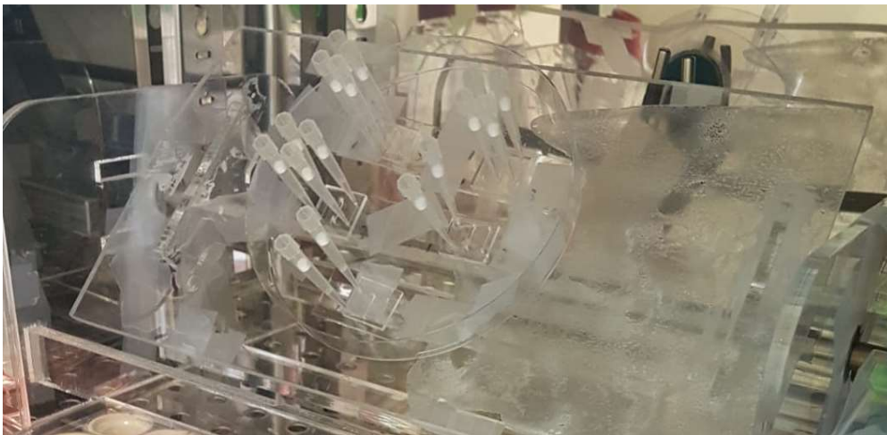
Figure 7: Cell-seeded chips on a see-saw rocker to create bidirectional flow. Rocker moves between +45 and -45 degrees to create a flow between the pipette tips filled with medium.
