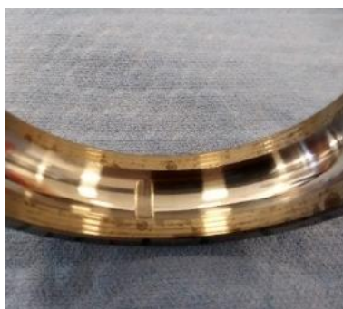
(a) 3mm spall
