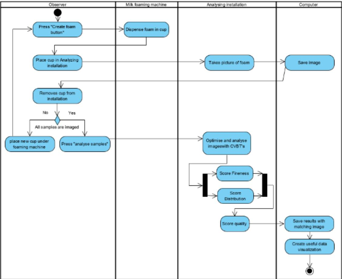
Figure 24 Workflow of preferred analysing method based on stakeholders' preference
