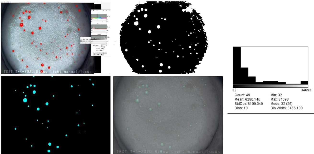
**Figure 30** *colour thresholding method in combination with particle analyses; a) manual colour thresholding; (b) binary image of colour thresholding result; (c) noise reduction + edge exclusion + particle analysis (d) overlaid result; (e) Bubble size distribution histogram after colour thresholding*
