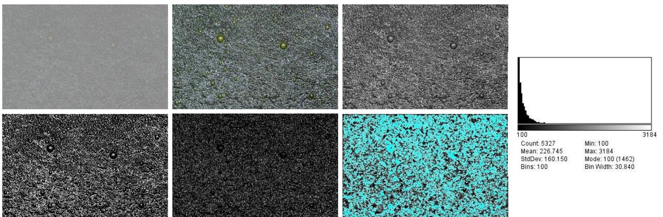
**Figure 29** *Result of literature based analysing method; (a) original sample (b) histogram equalisation (c) grey scaling (d) binary image (e) Canny edge detection + Watershed method (f) particle analysis (g) size distribution histogram*
