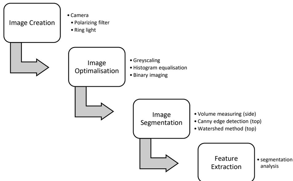
**Figure 15** *Workflow of optimized computer vision-based method to analyse bubble size and volume of milk foam based on the literature*
