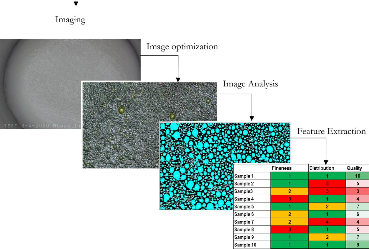
**Figure 8** *Visualisation of a standard computer vision based analysing method workflow*
