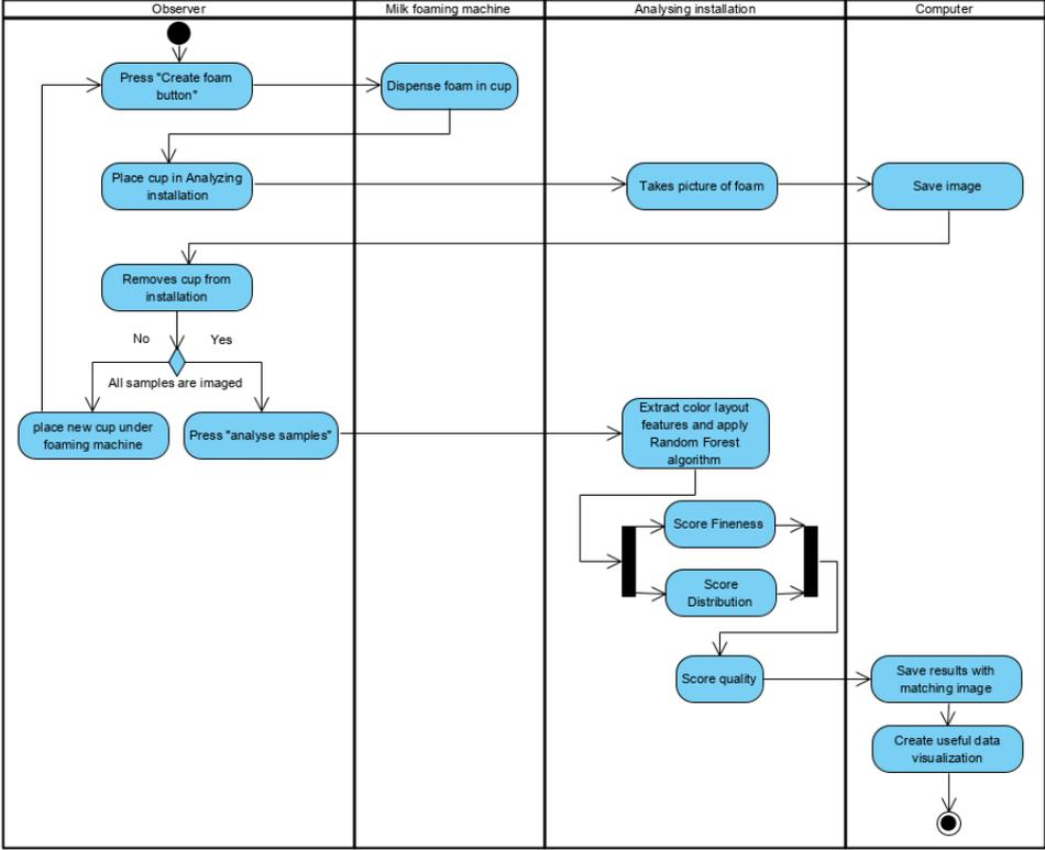
Figure 44 *Workflow of direct classification*
