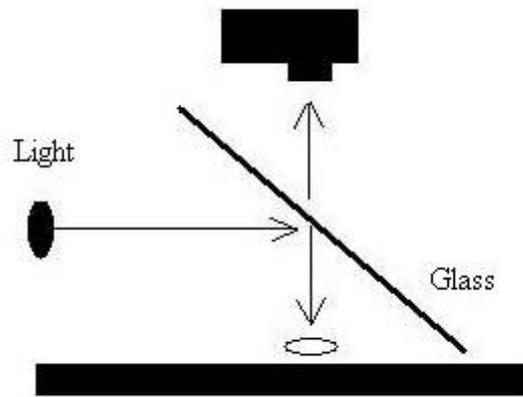
**Figure 34** *Axial lighting technique*
