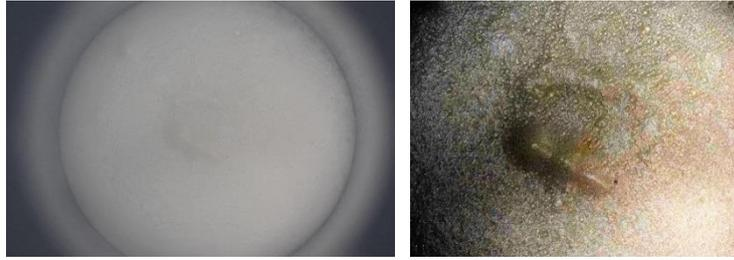
**Figure 33** *The use of multiple polarizing filters; a) the original image with 2 polarizing filter. (b) a sample of the centre of the image with histogram equalisation*
