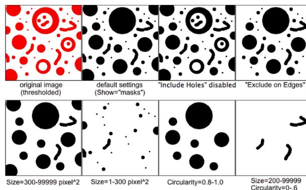
**Figure 22** *Particle analysis with Fiji*
