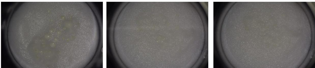
**Figure 36** *Minimizing light inconsistencies on sample a) normal b) with taped sides c) with taped sides and black cloth*
