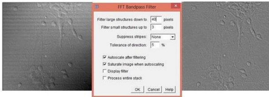
Figure 20 *Uneven background correction*
