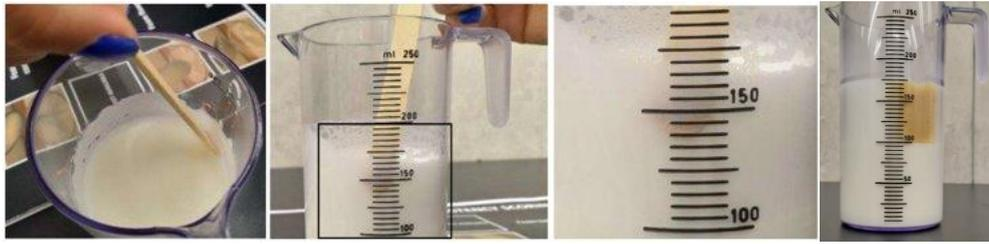
**Figure 5** *Volume measurements according to the milk scoring protocol*
