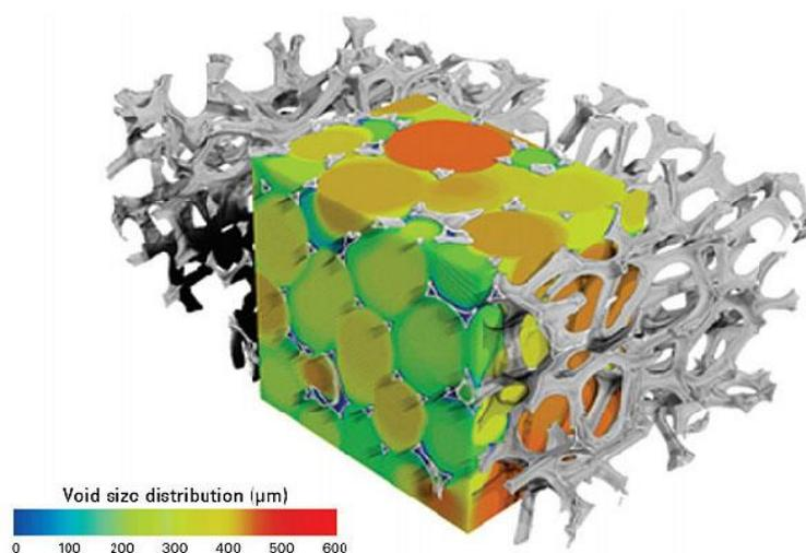
**Figure 18** *Micro-CT scan of a foam sample*
