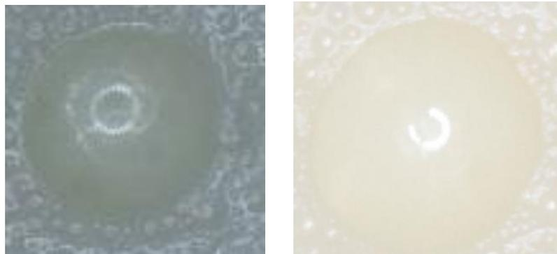
**Figure 32** *Ring light reflection in bubble a) normal b) with polarizing filter*
