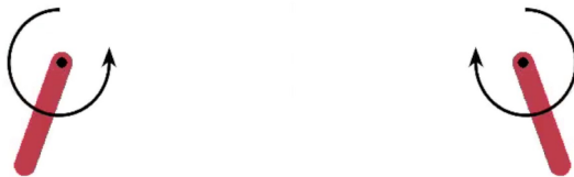
Figure 3: Example of state-action based data augmentation on a pendulum environment. Despite being two different states, the rewards obtained are equivalent if the actions are mirrored, effectively doubling the data that is available.
