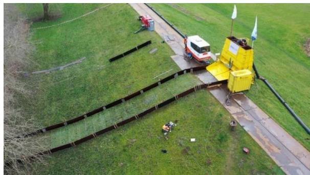
Figure 4: Setup of the wave overtopping simulator
