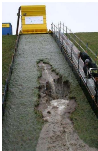
Figure 3: Erosion example caused by wave overtopping tests (Van der Meer, 2008)
