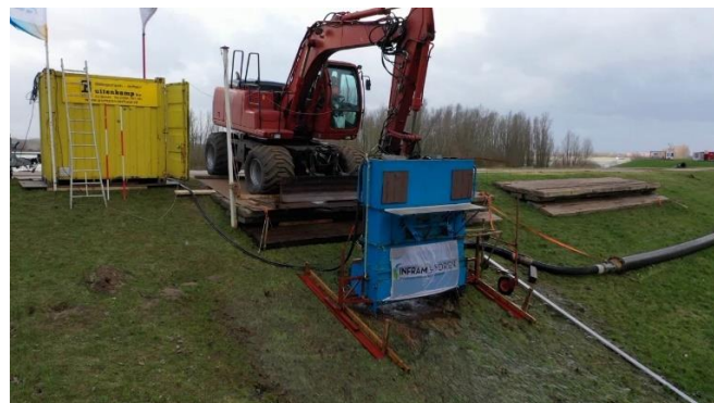
Figure 5: Setup of the wave impact generator
