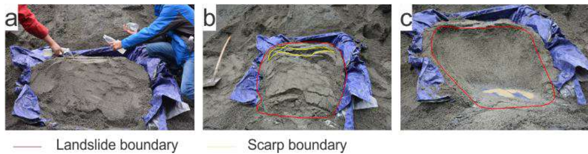
Figure 5: The experiment record of the deep-seated landslide. Figure (a) is the landscape before the failure, where (b) and (c) are after the failure and after digging the sliding material.
