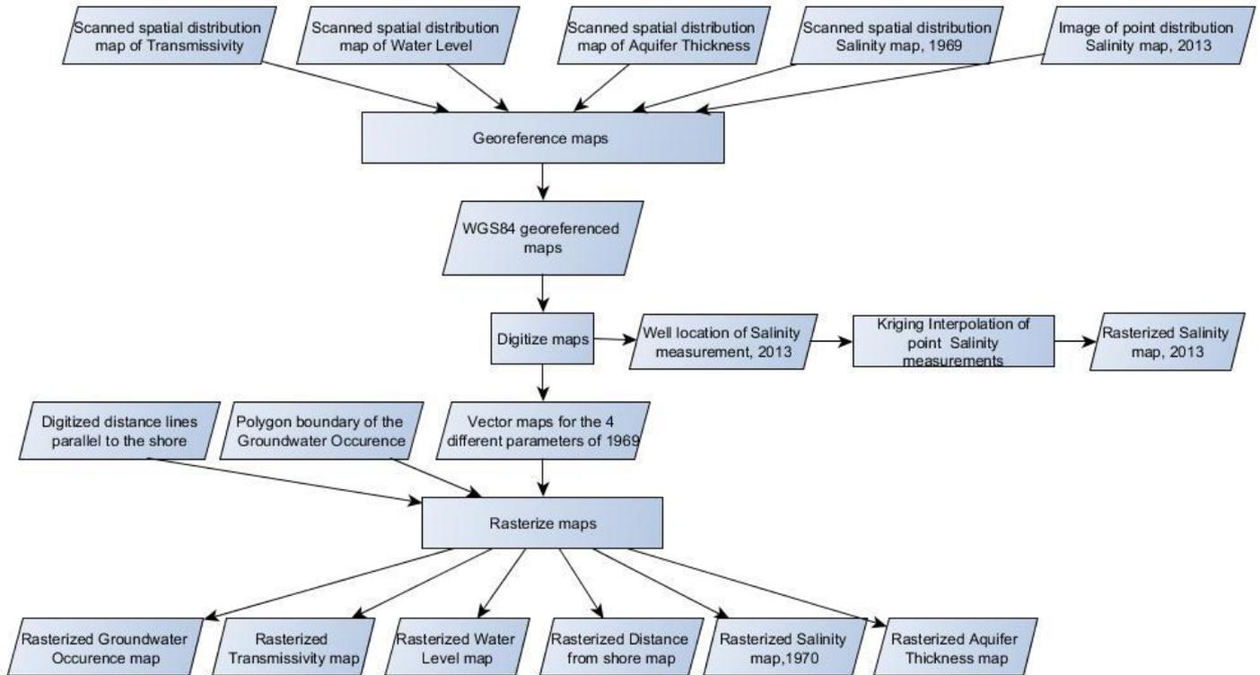
b-For processing Ghadir C4c data the below workflow is followed starting from digitizing the aquifer boundary from Ghadir formation map (Doummar et al., 2015). The processes used are: digitizing, overlaying, interpolating and rasterizing.
