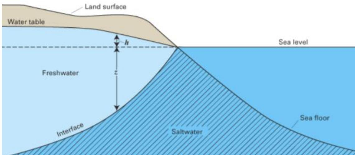
Figure 1: Hydrostatic equilibrium depicted by the sharp interface between freshwater and saltwater (Barlow, 2003).
