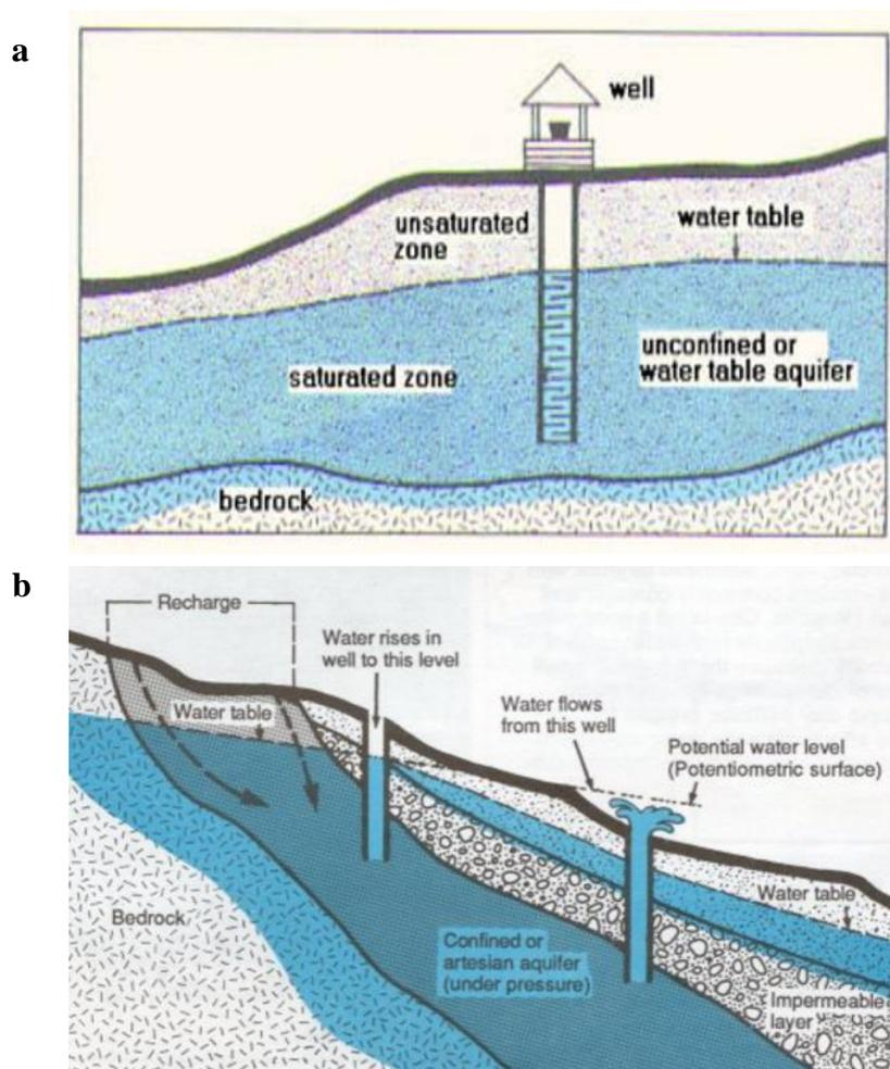
Figure 2: a) Showing an unconfined aquifer, where the saturated zone indicates the exploitable water zone, and the water table indicates water level. b) Showing a confined aquifer, and the recharge area that is not confined. The artesian well tapping the confined aquifer results from high pressure (Michigan Environmental Education Curriculum, n.d.).
