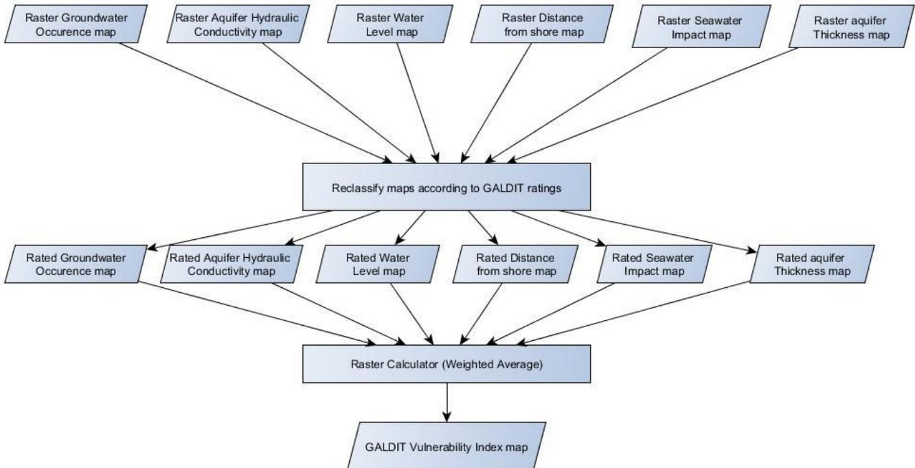
Figure 8: General workflow of GALDIT VI explaining the steps leading to the generation of GALDIT VI map, using the spatial distribution maps of the parameters as input.
