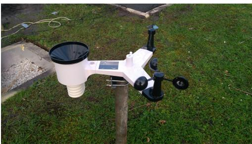
(a) WS-5500 weather station next to the setup to gather temperature, wind velocity and solar intensity data.
