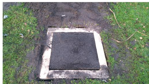
(b) Setup of 150mm foamed concrete and 80mm top layer, surround with isolation material.
