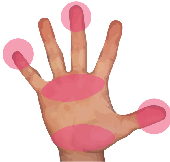
Figure 5.4: Pressure points on the hand that will be integrated into the design of the silicone inflatables
