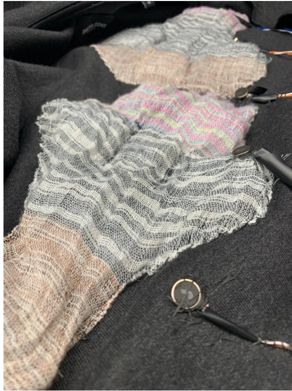
Figure 6.5: Close up of the silicone inflatables sown onto the wearable
