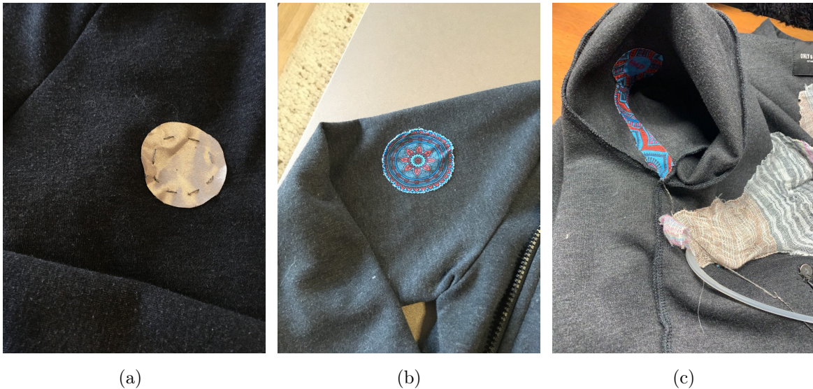
Figure 6.2: (a) Capacitive fabric sown onto the wearable, using conductive thread, (b) Capacitive sensor covered with regular fabric, (c) conductive thread on the inside covered with regular fabric.
