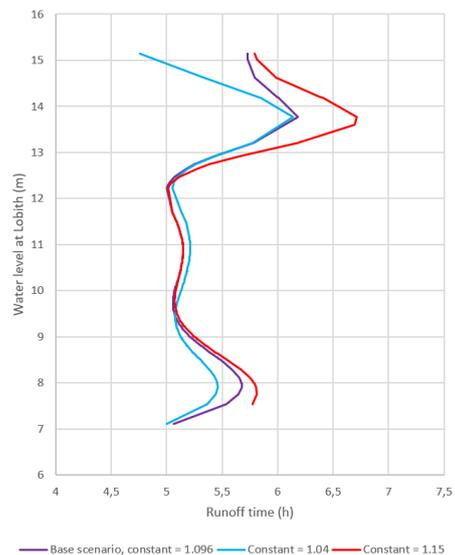
Figure 63 - Change of regression line by altering the distance underneath the peak at which the runoff time is determined
