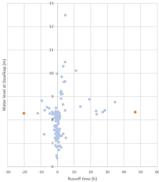
Figure 48 - Point cloud of water level valleys (IJsselkop – Driel boven, 2011 – 2019 data)
