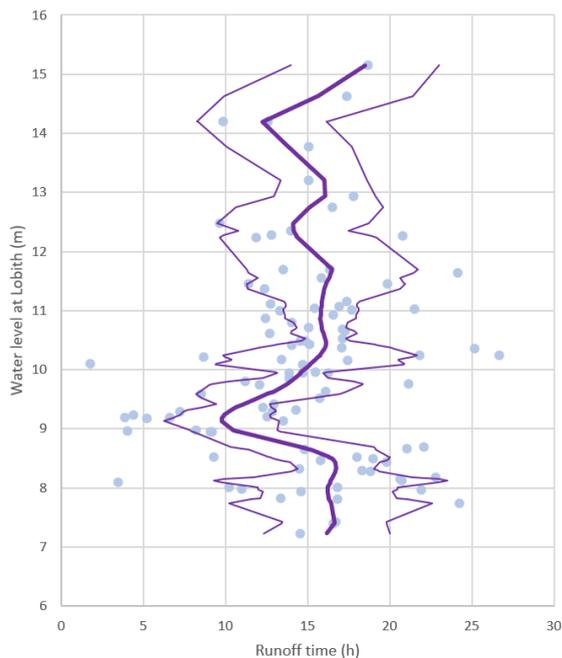
Figure 59 - Relation between runoff time and water level (Lobith - Doesburg, 2011 - 2019 data)
