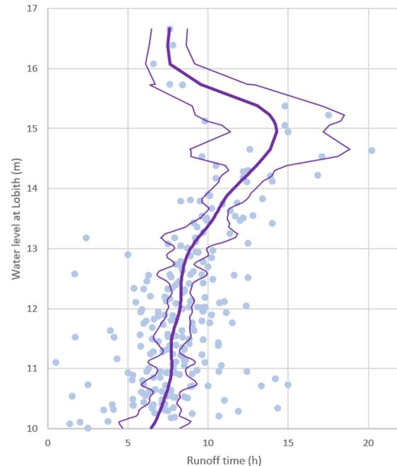
Figure 58 - Relation between runoff time and water level at high discharges (Lobith - Driel boven, 1985 - 2009 data)
