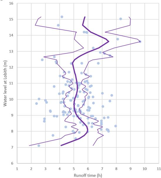
Figure 55 - Relation between runoff time and water level (Lobith - Nijmegen haven, 2011 - 2019 data)
