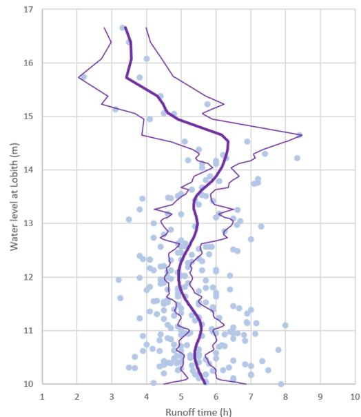
Figure 56 - Relation between runoff time and water level at high discharges (Lobith - Nijmegen haven, 1985 - 2009 data)
