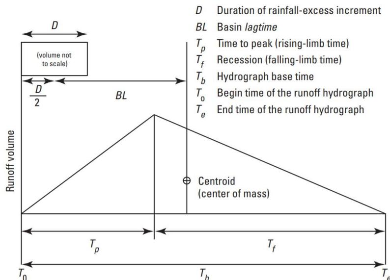
Figure 7 - Triangular hydrograph approach
