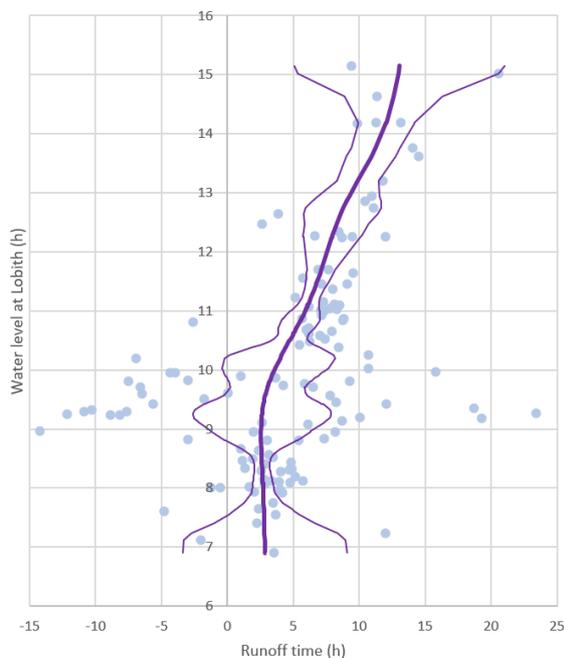
Figure 57 - Relation between runoff time and water level (Lobith - Driel boven, 2011 - 2019 data)
