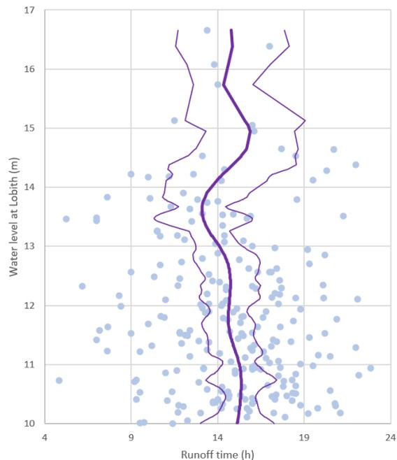
Figure 60 - Relation between runoff time and water level at high discharges (Lobith - Doesburg, 1985 - 2009 data)
