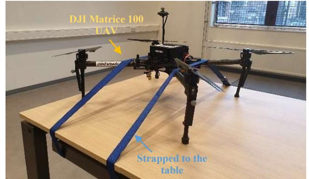
Fig. 31. DJI Matrice 100 UAV strapped to the table for safety purpose.
