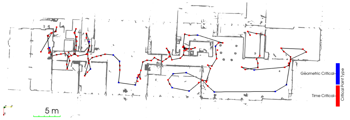
Figure 3.20: Merged critical points for the ZEB1 dataset top floor. Total of 143 critical points compared to 94,416 original points.
