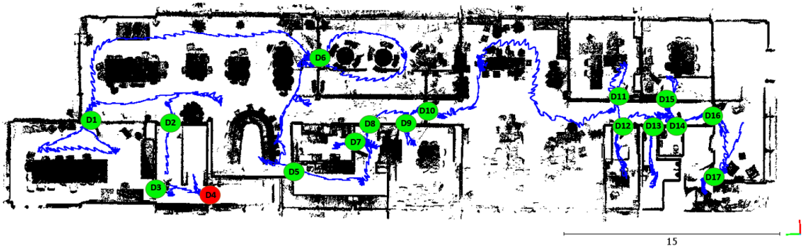
Figure 4.19: The top floor of ZEB1 dataset, the correctly detected doors are shown in green circles. Red circles represent the undetected doors.
