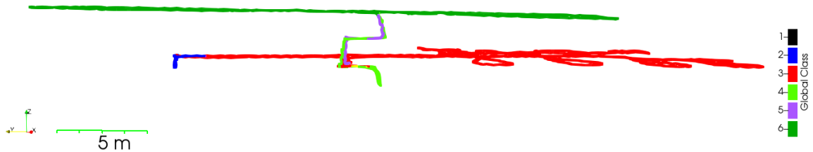
Figure 3.18: Global labels for ZEB-REVO dataset. Each global class represents a floor or staircase.
