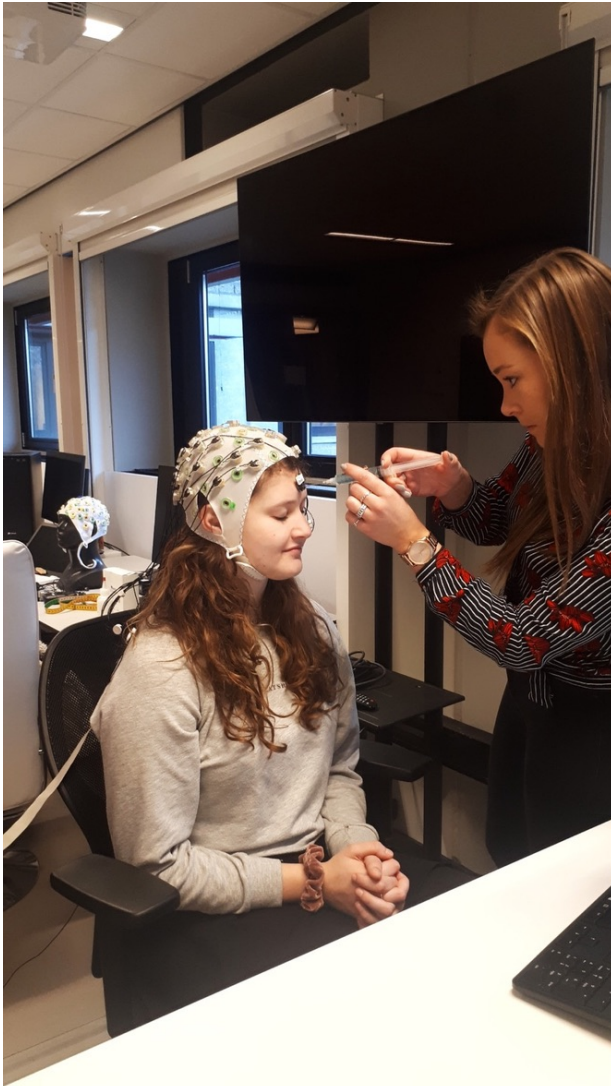
Figure F.1: The picture shows the researcher adding gel to the electrodes of the EEG cap a participant is wearing.*
