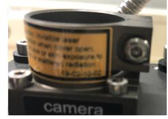
Figure 7.1: The compression fit linking the processing head and the optics.
