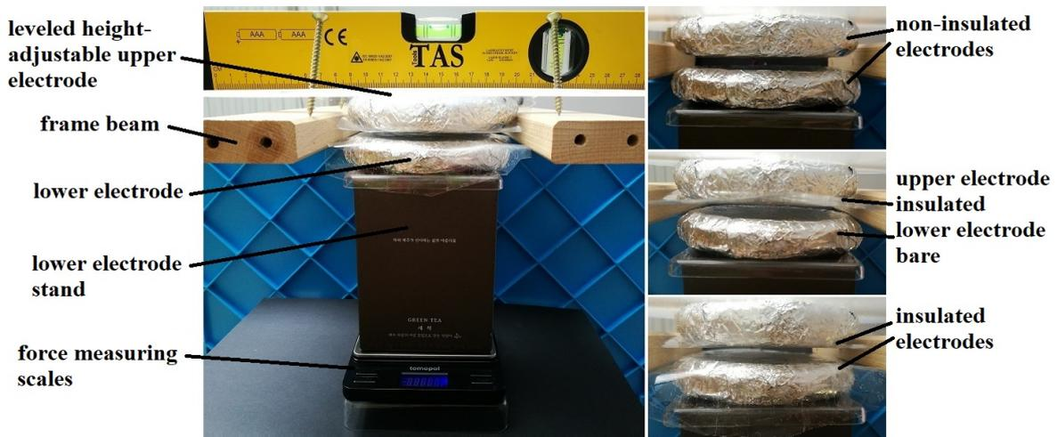
Figure 15: Overview of the components of the experimental setup
