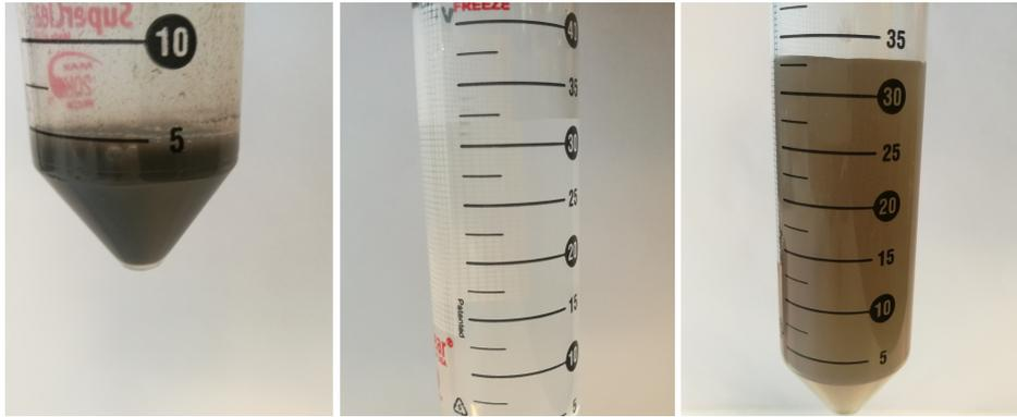
Figure 46: (left) concentrated collected contamination, (middle)  $32.2\text{ml}$  of purified water, (right) resulting  $33.2\text{ml}$  of twofold concentrated contamination fluid
