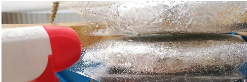
Figure 29: The insulated electrodes at a separation distance of  $3\text{mm}$  after water is sprayed into the gap
