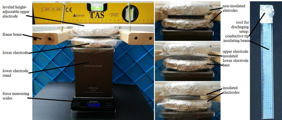
Figure 25: (left) The complete parallel capacitor force measuring setup, (middle) different electrode surface configurations from top to bottom: conducting-conducting, insulated-conducting, insulated-insulated, (right) electrode surface discharging tool
