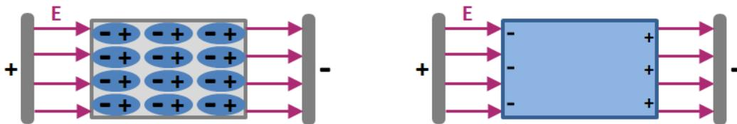
Figure 8: (left) Idealized dipole orientation withing a dielectric placed in a uniform electric field, (right) macroscopically resulting low level surface charge.
