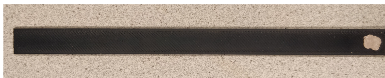
Figure 3.7: Picture of the sensor with same electrode size and X60 dielectric
