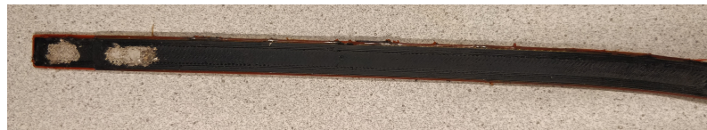
Figure 3.9: Picture of the differential sensor with NinjaFlex and X60 dielectric
