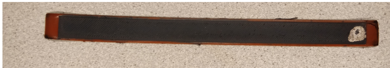
Figure 3.3: Picture of the sensor with NinjaFlex dielectric
