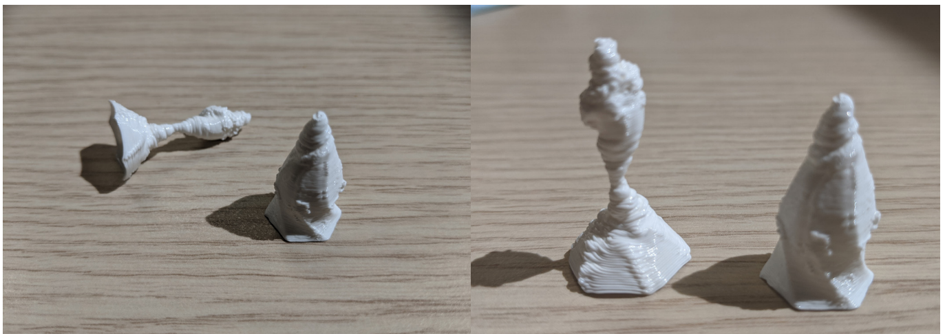
Figure 62: A design snapped in two during removal from the printer
