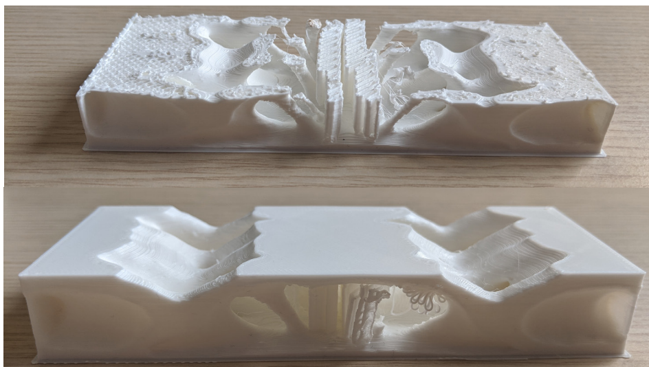
Figure 46: Two prints of the model above. They are the same but the first prints has been stopped midway the process
