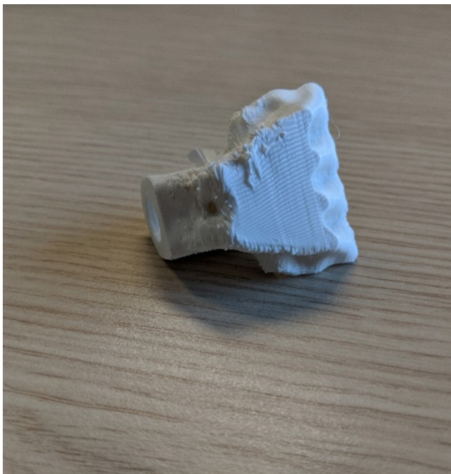
Figure 56: FDM result of previous figure in which support material is stuck in the part
