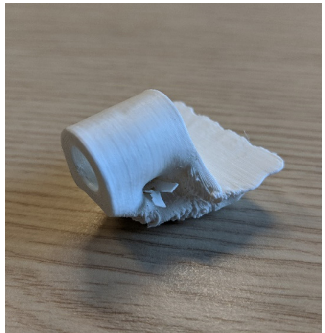
Figure 56: FDM result of previous figure in which support material is stuck in the part
