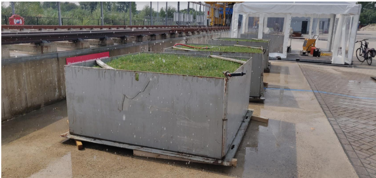
Figure 2-3 Clay blocks with grass and steel moulds as used in the Deltares delta flume experiments.
