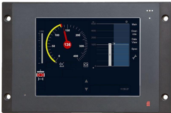
Figure 2.3: Example of a Driver Machine Interface (ERSA by CLEARSY, 2021)
