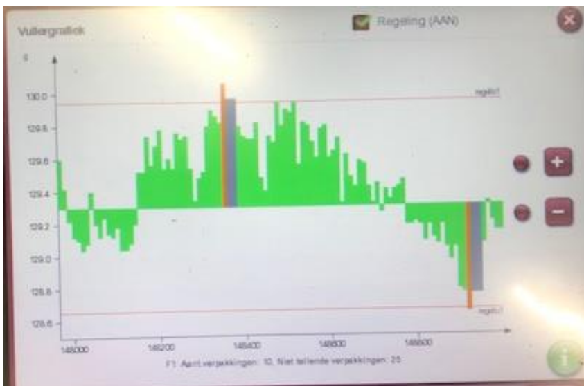
FIGURE 16: EXAMPLE OF FLUCTUATION OF FILLED PRODUCT CARRIER WEIGHT BETWEEN THE TOLERANCES OF \pm 0.7 GRAMS (PHOTO TAKEN FROM LINE 17, NOT POSSIBLE TO TAKE A SCREENSHOT).
