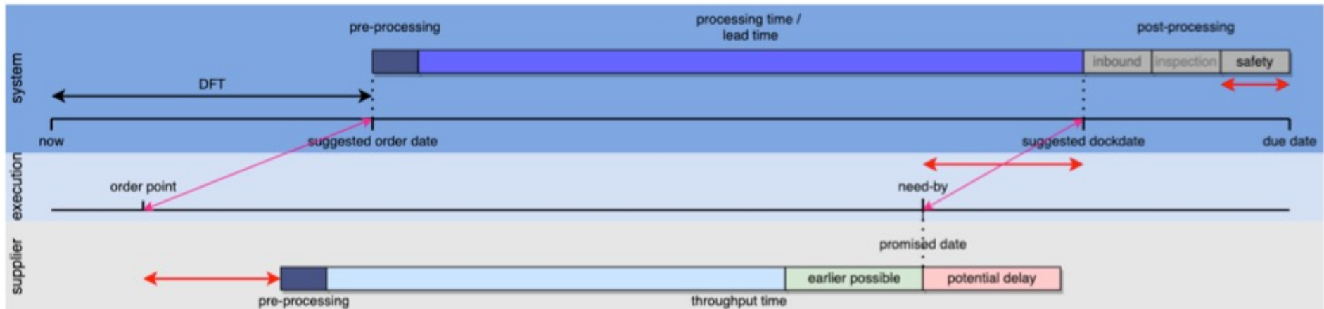
Figure 21: Overview of lead times in current situation, with buffers indicated in red and misalignments indicated in pink.
